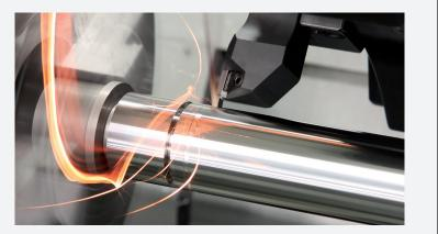
The new PcBN grades minimize chipping of PcBN tool edges by the strong bonding effect of proprietary CBN powder processing technology. And show reduced crater wear due to new developed ceramic binder systems which increased the hardness and heat resistance. The products are designed for processing various heat-treated steel parts and will provide improved workpiece surface quality and tool life.
